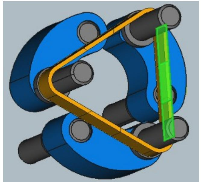
We can now simulate the deformation of the elastic and the movement of the flyweights :
