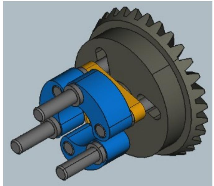
**Note** : It is normal that there is no longer any mobility because the **elast\_masselottes** part is actually an elastic which limits the centrifugal effect on the weights, and of course here this object is not deformable.
